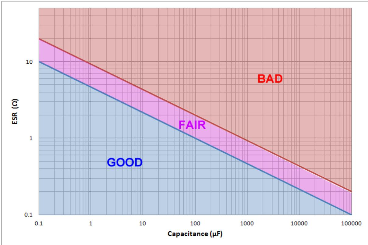
Figure 1 - Relationship between capacitor condition, capacitance and ESR
