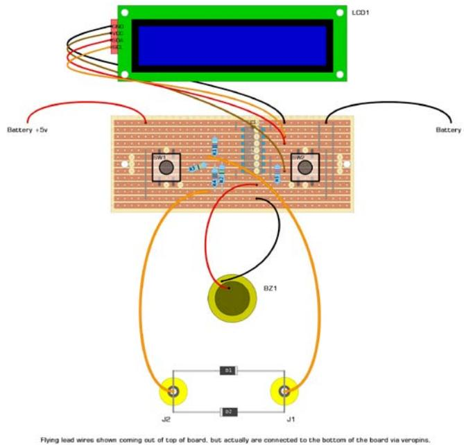
Figure 4 - Wiring components to the main-board
