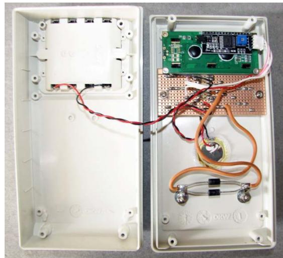
**Photo 2 - Mounting components in the DATEC-MOBIL-BOX enclosure**
