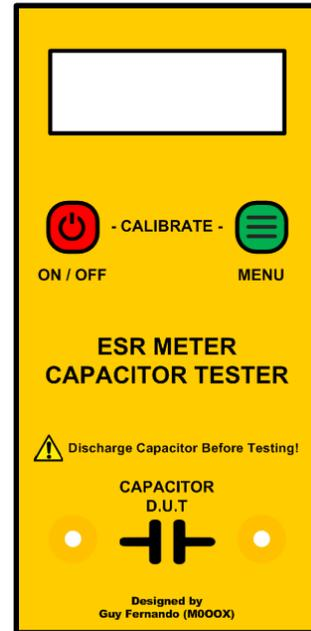
Figure 5 - Front panel artwork (80mm x 167mm)
